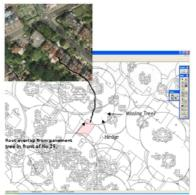
The modelled root zone suggests that the pavement tree is the most likely cause of damage when root zones are plotted.
